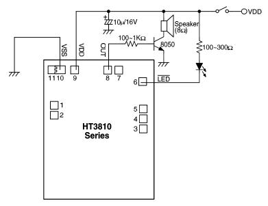
$\ast$  The substrate should be connected to VDD in the PCB layout artwork.
