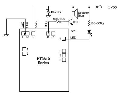
\* The substrate should be connected to VDD in the PCB layout artwork.
